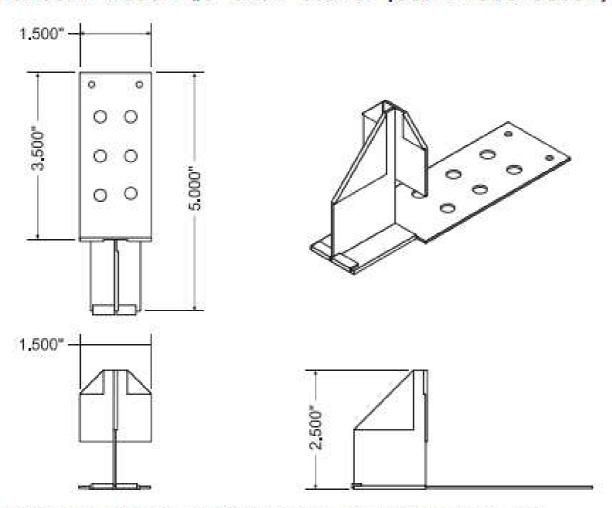
MATERIAL: Our model No.-9 Snow-Guard is manufactured using .020 thickness of stainless steel. Since it is double thick the result is .020  $\times$  2 = .040.
