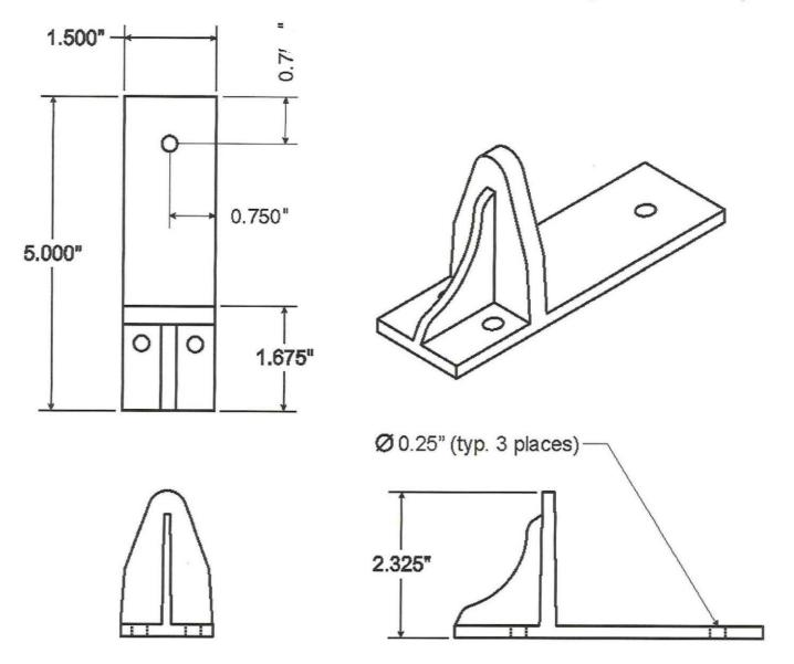
MATERIAL: Our model No. 11-A Snow-Guard is manufactured using #319 aluminum for casting. Tensile strength 17,000 pounds per square inch. We offer a baked on painted finish to match your color sample.
